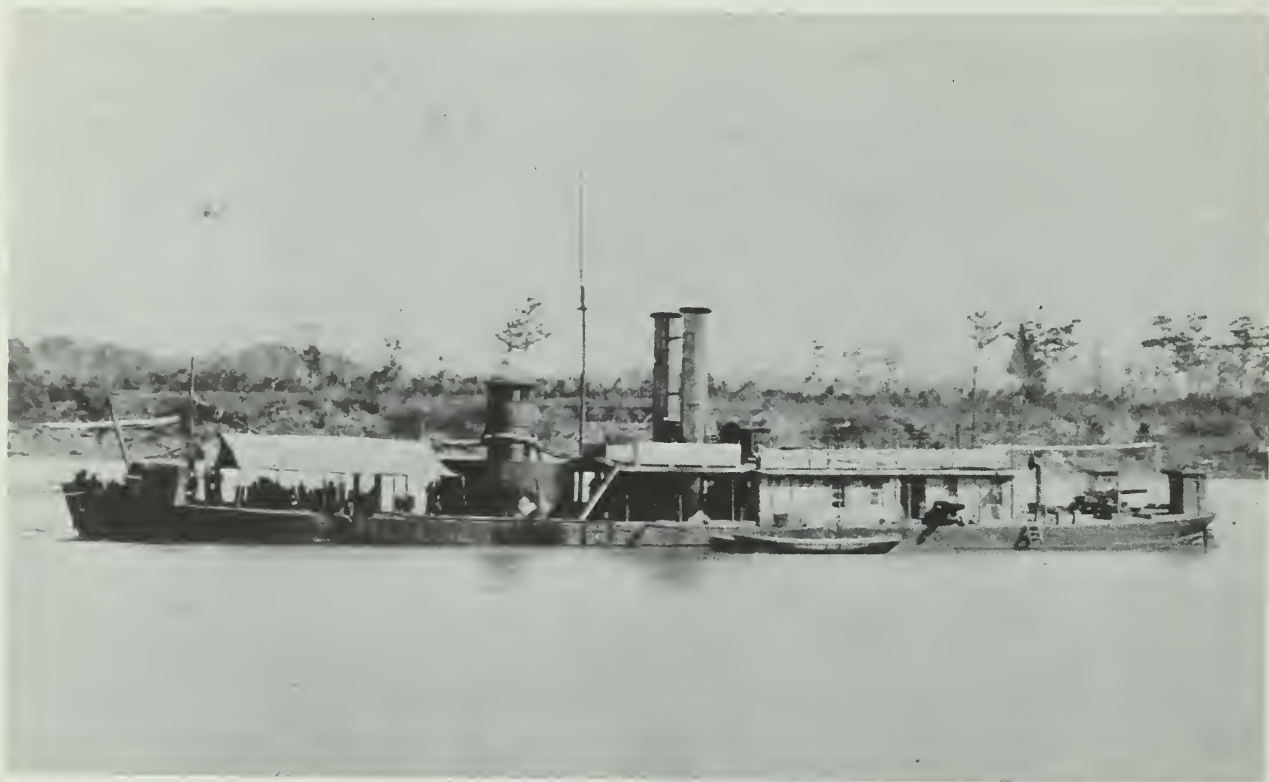
U.S. Monitor Ozark while part of the Mississippi Squadron in 1864—The deckhouse and exposed pivot guns may be seen clearly. USS Ozark 's pilothouse resembles that which was placed on the main deck of the Milwaukee class. The pilothouse on most monitors was approximately 6 feet high but that on USS Ozark appears to be about 12 feet in height.
